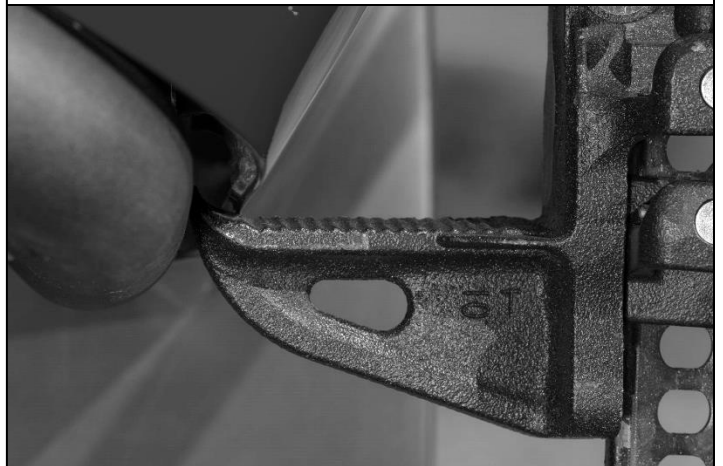
HIGH LIFT JACK LOCATION - SIDE OF WING/ABOVE TUBE
